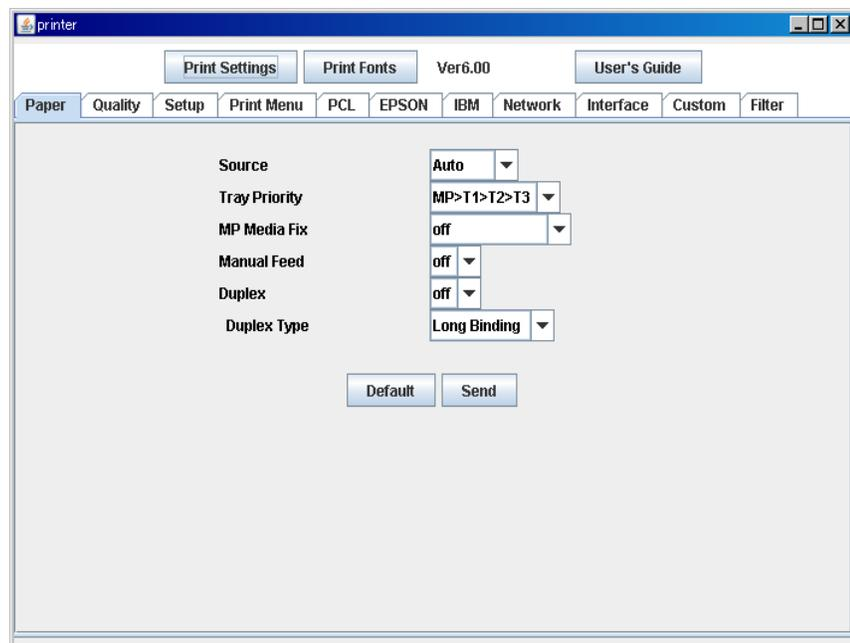
The Remote Printer Console is a software utility for changing printer settings independently of your software application. For example, you can change the printer margins, sleep mode, character set and other settings from the Remote Printer Console software. These settings are then remembered and used by the printer.
